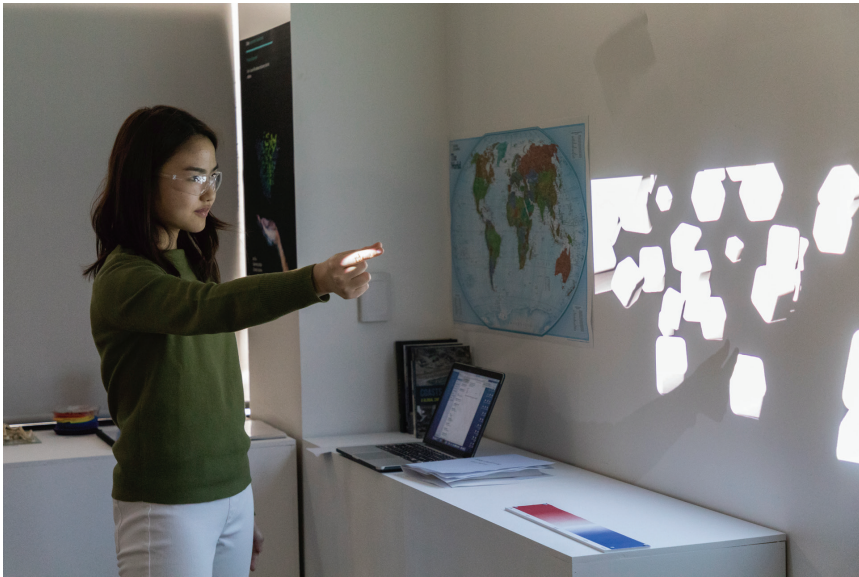
Figure 8. When researchers put on the AR glasses, they can visualize the eddy from different viewpoints and filter out specific factors. Using large gestures (grab, swipe, pinch, rotate, etc.), they can separate layers, zoom and track, push away and push to save the results
