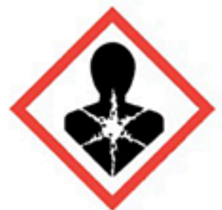
vakava terveysvaara serious health hazard
